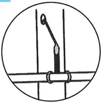
Use items like door frames, eyelets and "u" channels to secure hose with hangers. *Take up slack.*
