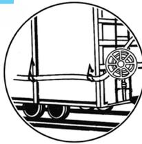
Walk lead end of hose along car. Shut cut-out cocks at both ends of adjoining cars.
