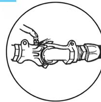
To remove: use vent valves on the Run-A-Round hose gladhands to bleed excess air before disconnecting manually.
