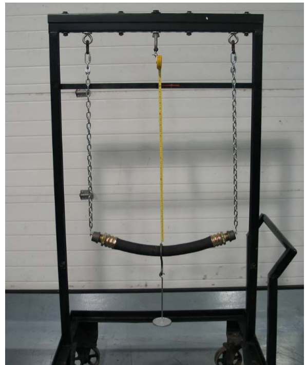
Figure 1: Test Fixture photo, Former SUSPENSION Test Method, Male x Male, Cold Room
