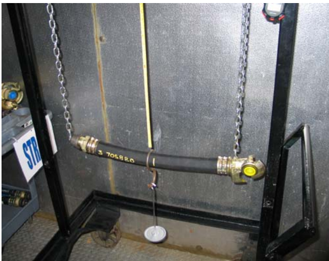
Figure 1B: Test Fixture photo, Former Proposed SUSPENSION Method, Male x Gladhand, Cold Room
