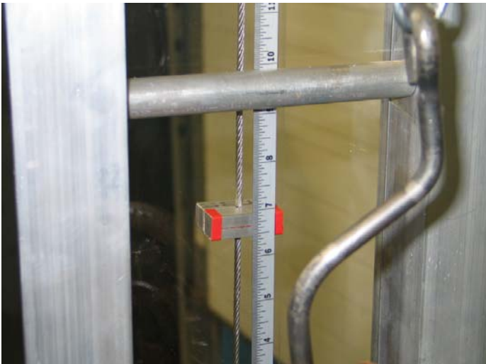
Figure 5A: Shows scale on Flex Device for measuring deflection
