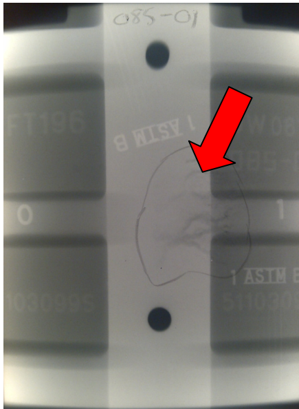
Figure 7: Radiographic Image Showing Level 5 Shrinkage.
