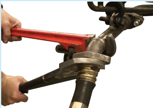
End hose removal is difficult when using double wrenches
