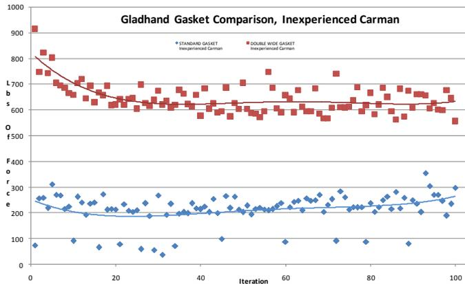
FIGURE 7: STANDARD VS. DOUBLE WIDE, PULL APART FORCE
