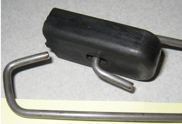
Figure 8: Previous design, failure always occurred at location closer to the opposite end
