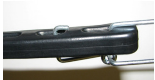
Figure 10: Side view of dual-leg metal hook engaged with rubber strap under medium load condition
