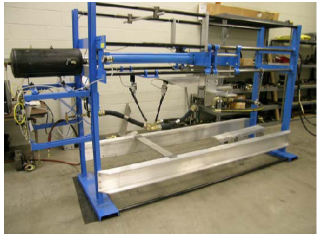
Figure 2: Device for simulating end hose arrangement. Hose support straps are connected to a set of load cells to monitor tensile force.
