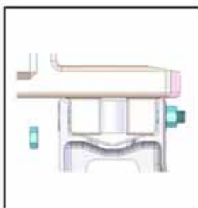
1.) CUT HEAD OFF OF OLD BOLT.
